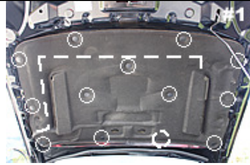
Remove circled pins. Route wiring along dashed line.
