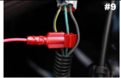
Plug red wire into the wire tap as shown. 2013-14 Connector shown.
