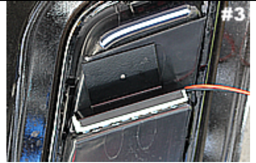
Shown is the passenger side turn signal mounted to the heat extractor.
