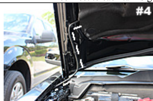
Use zip ties to secure wiring at hood base – follow washer fluid hose.
