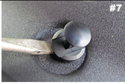
Pry up on center part of pin first. Then pry out entire retainer pin.
