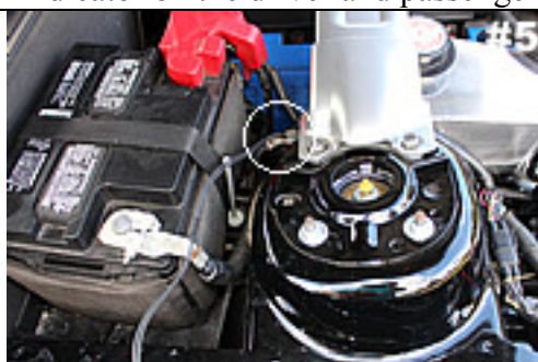
Attach ring terminal to bolt circled above or nearby. Re-tighten the bolt.
