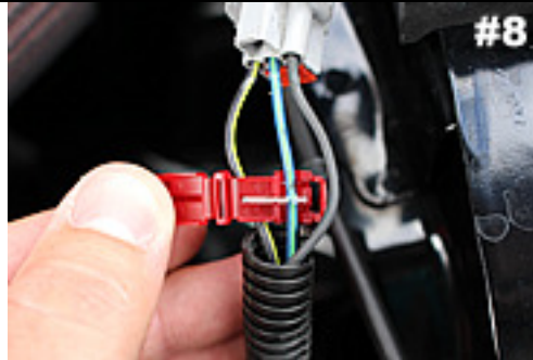
Slide wire into place and close wire tap. 2013-14 Connector shown.
