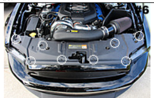
Remove black panel shown. Save retaining pins for re-install later.
