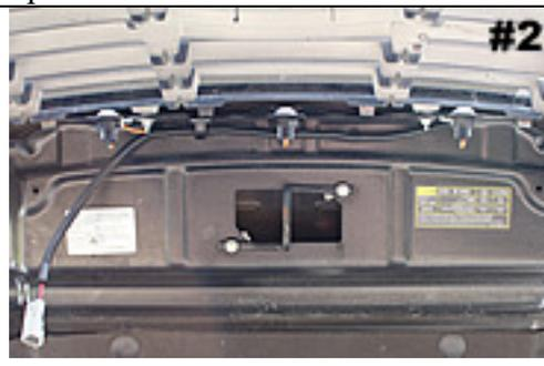
Position bracket and tighten the 10mm nuts.
