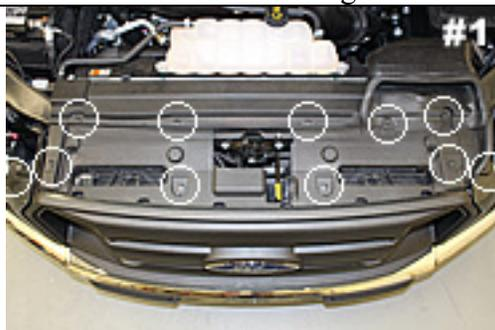
Remove black panel shown. Save 11 retaining pins for re-install later.
