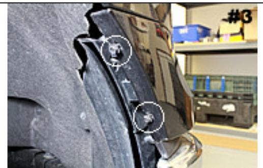
Remove 2 - 7mm bolts on driver and passenger side wheel well.
