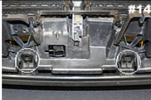
Use the 2 of the large push-pins to secure the L-brackets.
