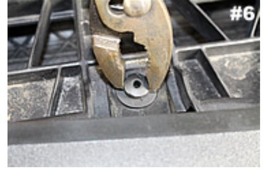
Use pliers to pull the large push-pins straight up and out of grille.
