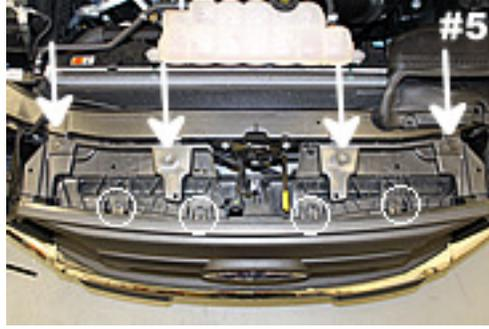
Remove 4 – 10mm bolts and then remove 4 push-pins circled above.
