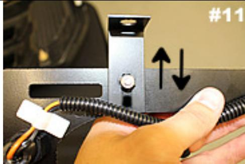
Slide L-Bracket up or down to adjust height of light bar. Then tighten nuts.
