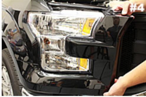
Remove headlight trim starting at inside top and finish at wheel well.
