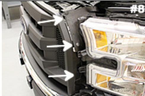
Remove the 6 push-pins holding rubber shield to grille. 3 on each side.
