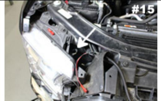
Locate the amber running light connector behind the head light.
