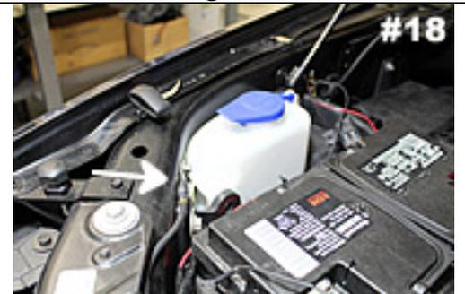
Attach the ground wire to the bolt in front of washer fluid reservoir.
