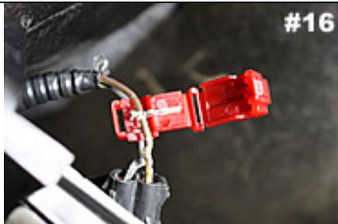
Slide wire into place and close wire tap completely.
