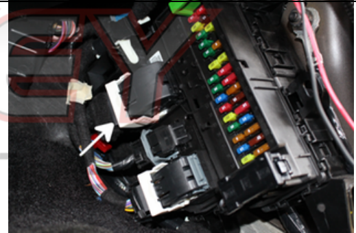
Press tab while sliding bar to the side to unplug connector. 4
