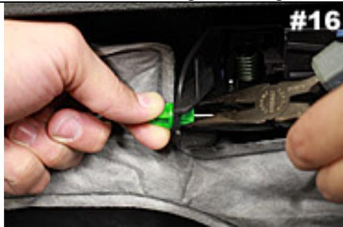
Use a pair of needle nose pliers to remove door handle cable.
