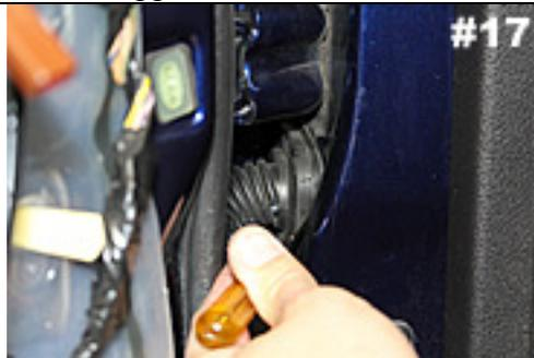
Loosen the rubber boot in the door jamb but do not remove it.
