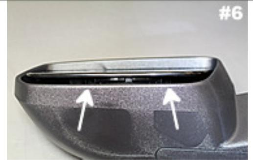
Bottom view of Drivers side mirror. Shown are 2 of the retaining tabs.
