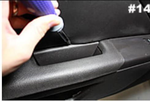
Remove trim piece and Torx T30 screw behind the arm rest.
