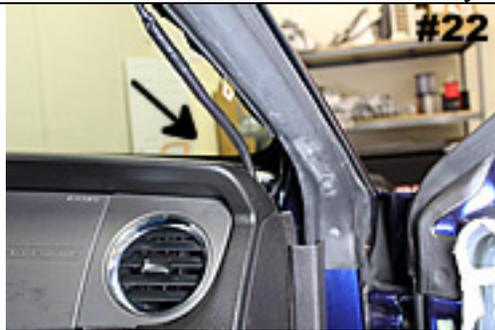
Run wiring harness through gap near a-pillar to passenger side floor
