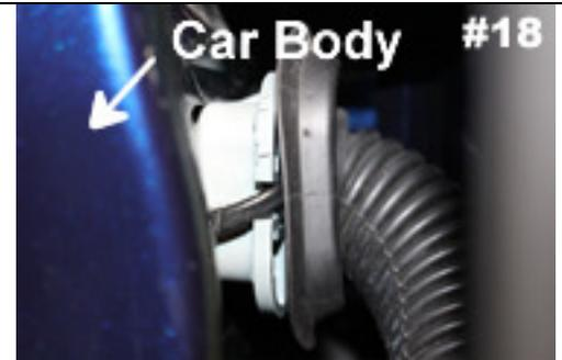
Loosen connector by depressing top & bottom tabs and pulling 1/2 inch out.
