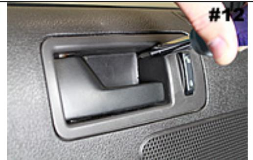
Remove trim panel behind the door handle with flat head screwdriver.
