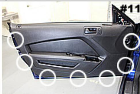
Remove screws around perimeter of door with 7mm driver.
