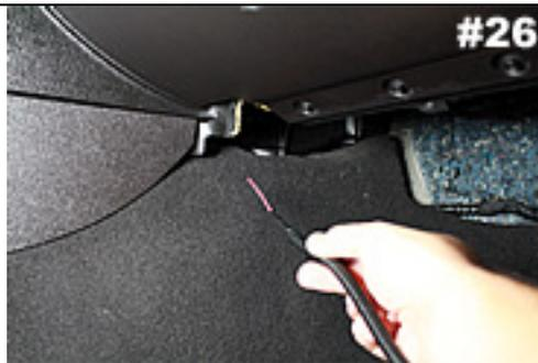
Pass remaining wiring behind center console to drivers side.
