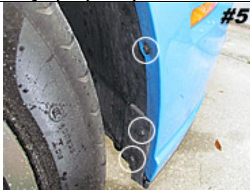
Remove 3 bolts on driver and passenger side wheel well.
