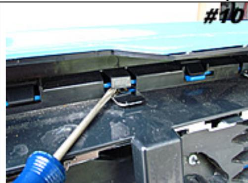
Top row of tabs shown. Pry up with screwdriver while pushing tab down.
