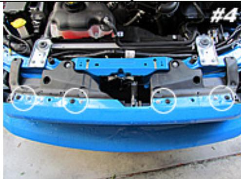
Remove 4 bolts (8mm) and 4 push-pin Phillips screws.
