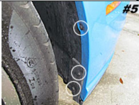
Remove 3 bolts on driver and passenger side wheel well.
