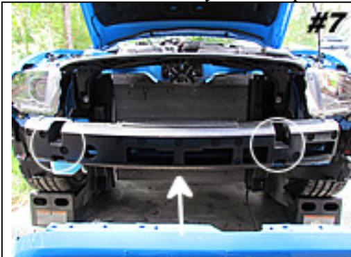
Re-attach black Styrofoam piece with 4 ribbed push pins before continuing.
