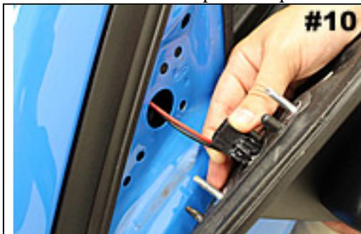
Lamp wiring goes through same hole as the mirror's electrical connector.
