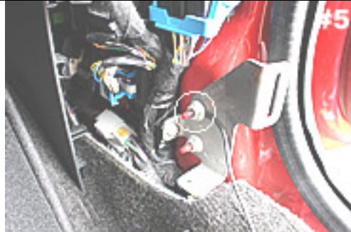
Attach black ground wire to the 10mm bolt circled above.
