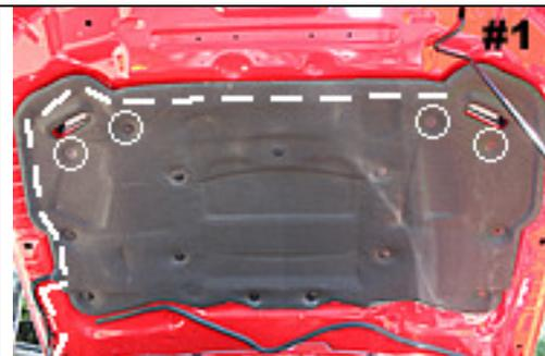
Remove 4 circled pins. Route wiring along dashed line.
